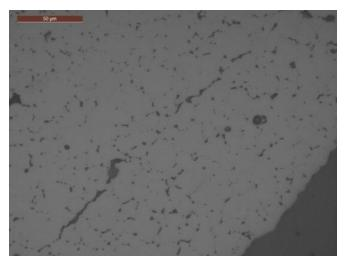
c) High magnification micrograph showing plentiful intergranular porosity, with some interlinking.
