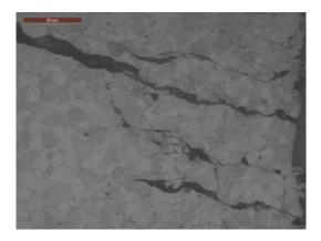
(a) Fuel cracking
