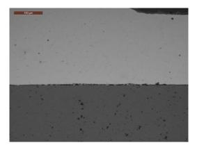
Figure 13: As polished image showing the fuel-clad gap in 424/4.
