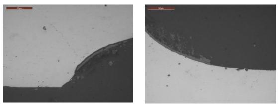
(a) Oxide(b) Carbon depositFigure 7: Rib roots showing the remains of oxide and carbon deposit (221B/4).
