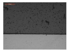
Figure 6: As-polished micrograph showing the continuous fuel-clad gap found on 221B/4.
