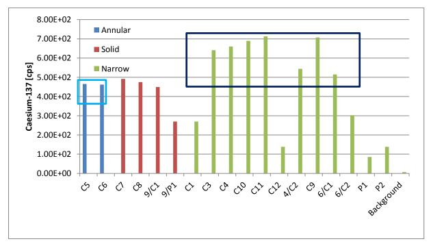
Figure 2. Spot gamma scan results for retained fuel pins
