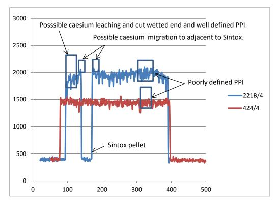
Figure 3. Axial gamma scan of pin sections examined.
