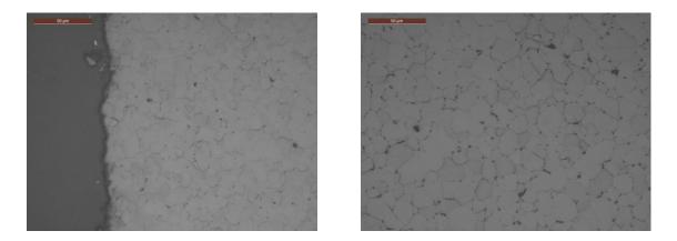
Figure 22: IE 424/4 – Etched micrographs of the fuel at the non-wetted end.
