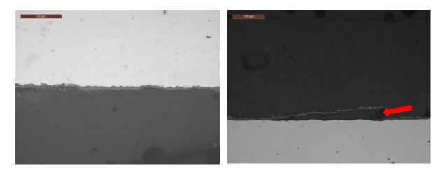
(a) Typical clad outer surface oxide layer
