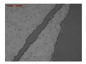
(b)Fuel crack within the region where the fuel was missing
