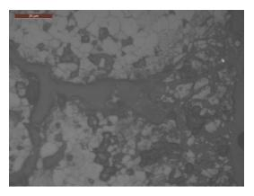
(b) Sintering defect
