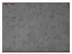
(c) Intergranular porosity Figure 23: IE 424/4 – Etched micrographs of the fuel at the wetted end.
