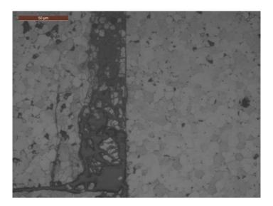
Figure 26: IE 424/4 – Etched micrograph of the PPI within rib space L.
