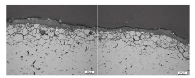
Figure 1. A cross sectional image through an irradiated fuel fragment exposed to simulated ground water (Zwicky, Low, & Ekeroth, 2011).
